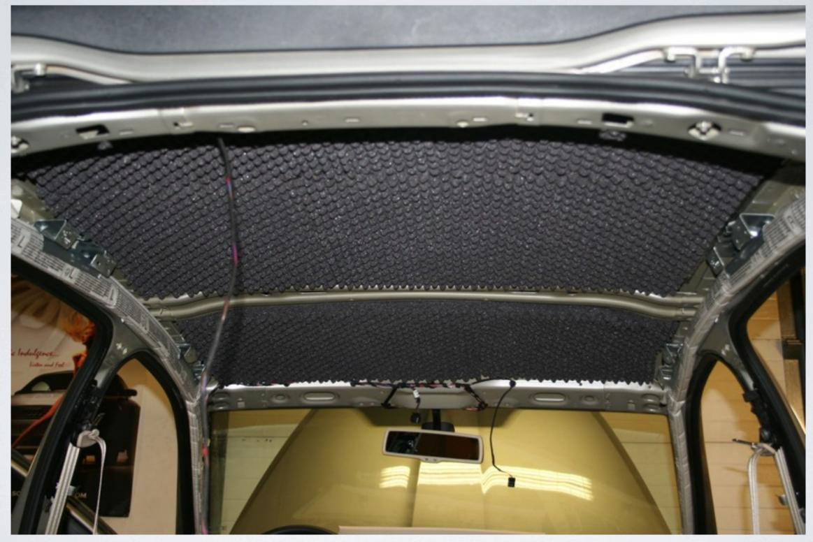
Combination of Silent Coat and Absorber 35 is used for the roof.
